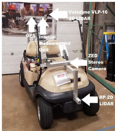
Figure 5. Approximate Sensor Placement
