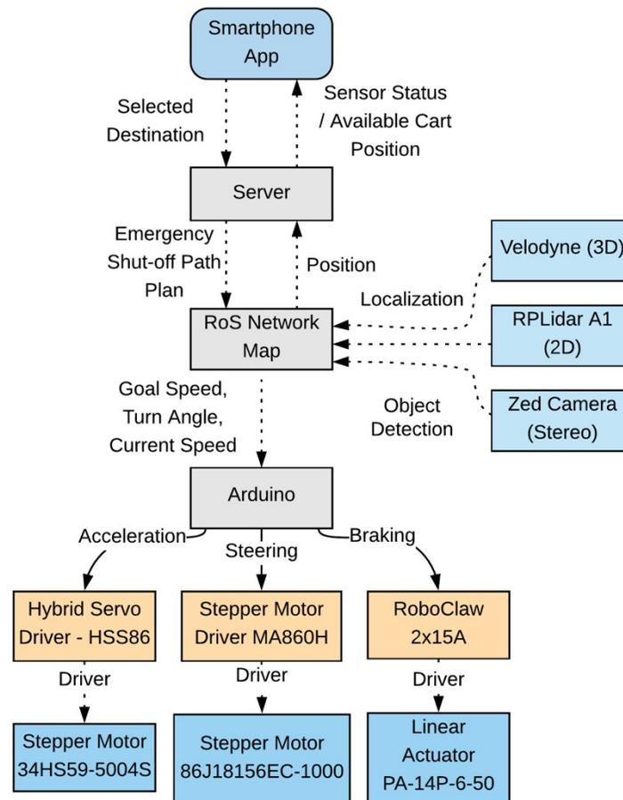
Figure 2. Technical Data Flow Diagram
